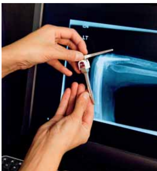
Special Surgery biomechanical engineers compare retrieved elbow implants with x-rays to learn how elbow implants work and how they can be improved.
