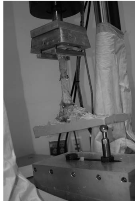
Fig. 2: This specimen, stabilized with an IM nail, is seen here in the dorsiflexion testing set-up with an unconstrained fulcrum under the distal foot. Angular displacements were calculated from local motion measurements recorded in this position.
